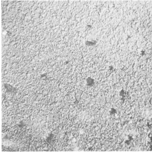
Figure 4 Microstructure of magnesium-doped beta-alumina showing fine grain structure and substantial absence of coarse grains, \times 750
